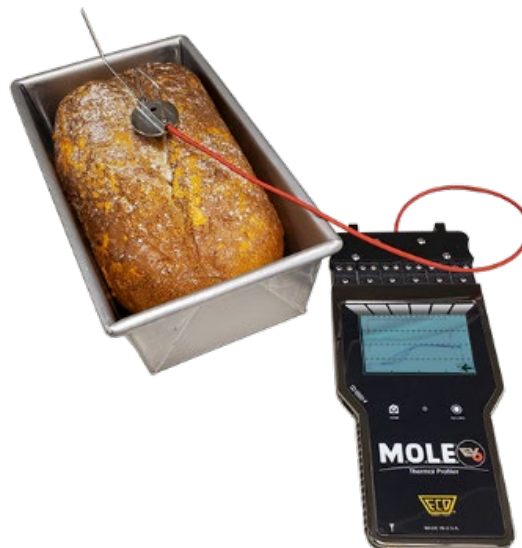
Figure 5: The BreadOMETER simplifies S-curve management with a patented all-in-one sensor design, allowing a single probe insertion for multi-depth dough measurements. The ambient sensor measures accurate oven line and delineates oven entrance and exit. The M.O.L.E. EV6 touchscreen thermal profiler displays S-Curve data and allows control from the handheld device; no PC download is required to view the profile
