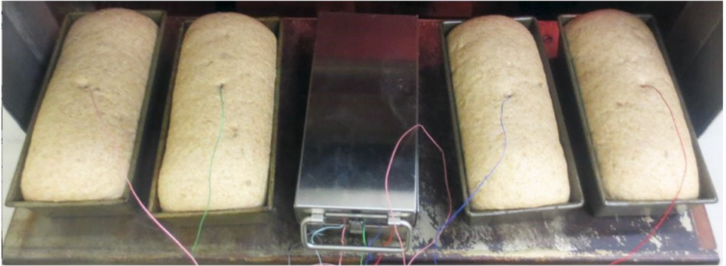
Figure 4: Multiple runs are typically required across the oven to discern if the oven is balanced left-to-right across the conveyor, or if it's consistent between upper, middle, and lower shelves. Variations in thermocouple sensor placement (i.e., location, depth, angle, etc.) and even dough placement in the oven can also cause alterations in the data. There are models available, like the BreadOMETER from ECD , that have fixed positions for the ambient and insertion sensors up to the stop plate.
