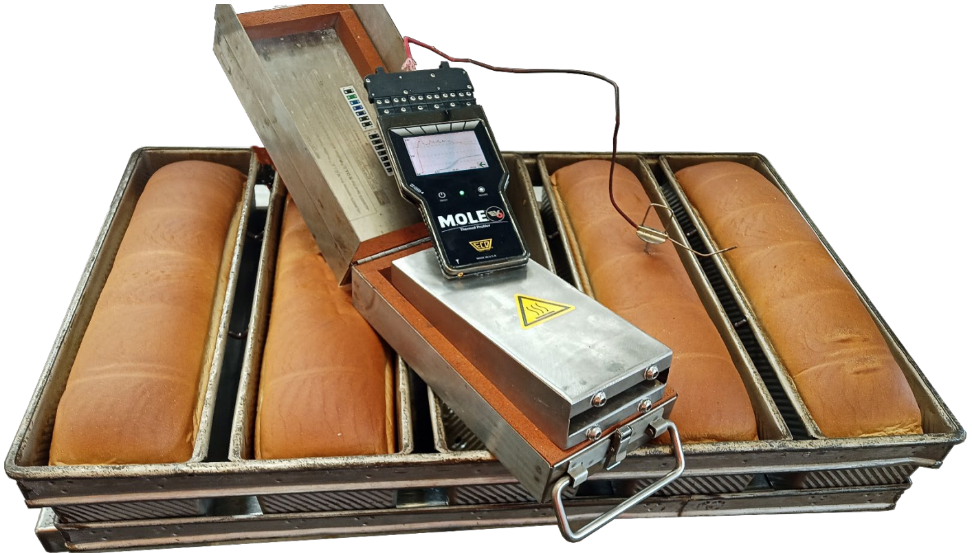
Figure 6: Thermal profiler innovation with touchscreen M.O.L.E. EV6 allows S-curve viewing and data-informed process adjustments on the fly. No PC download is required for data viewing and analysis.
