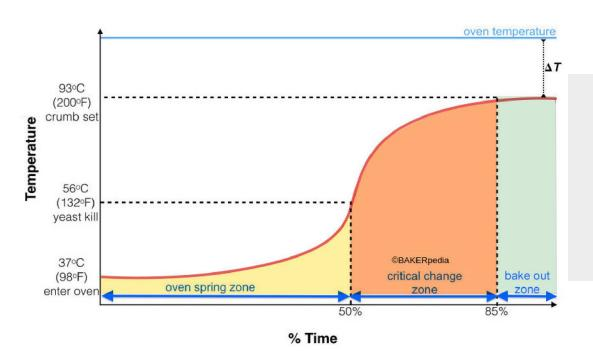
In this example, the product is maintained at 37°C(98°F) for optimum fermentation output. The internal product temperature rises in the oven as it moves inside in a continuous oven system and the product passes through all three phases.
