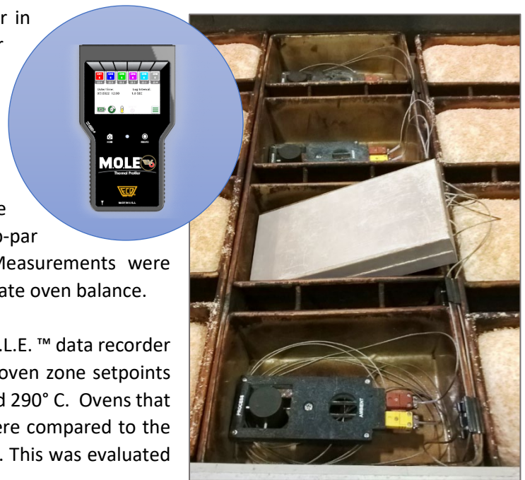
Figure 2: OvenBALANCER sensors are placed in loaf pans and a M.O.L.E. EV6 (inside the center barrier) collects in-process temperature data.
